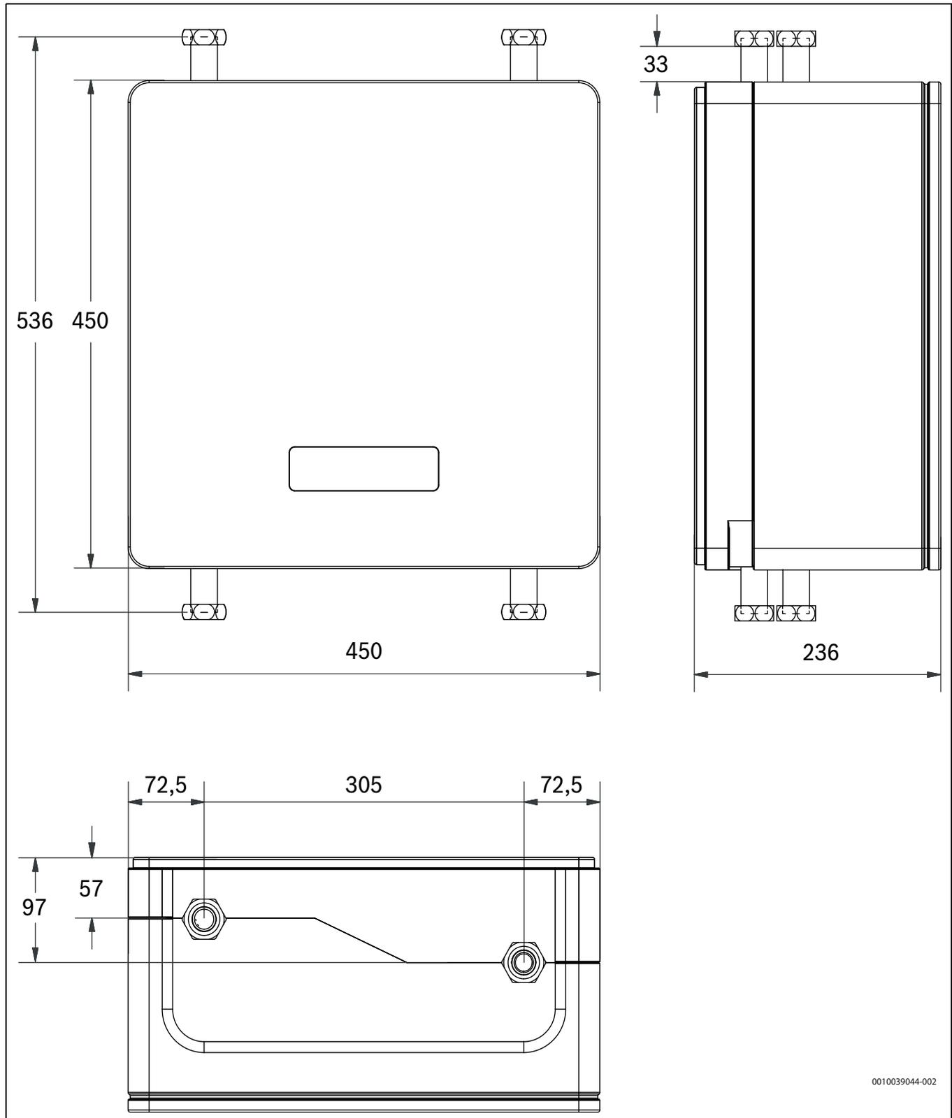
Fig. 3 Dimensions, raccords
